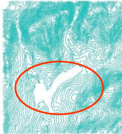
Contours after filling the pits
